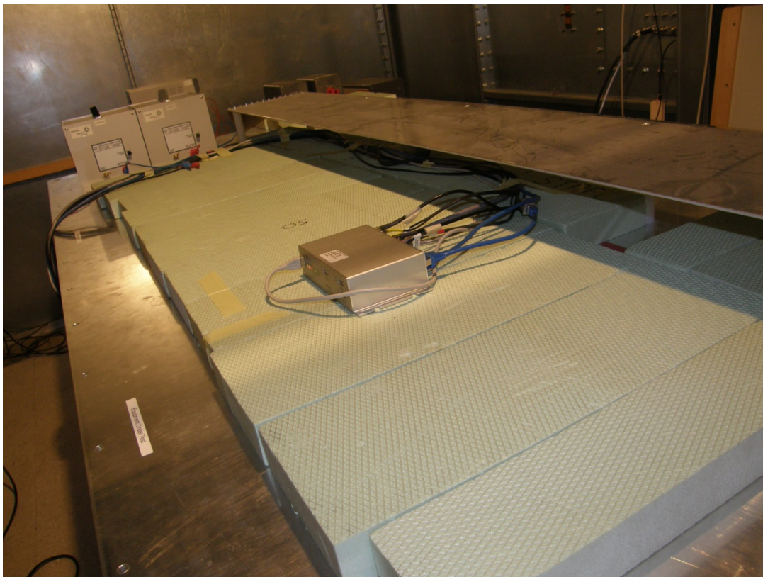
Photo 13: Set-up for the Stripline test
